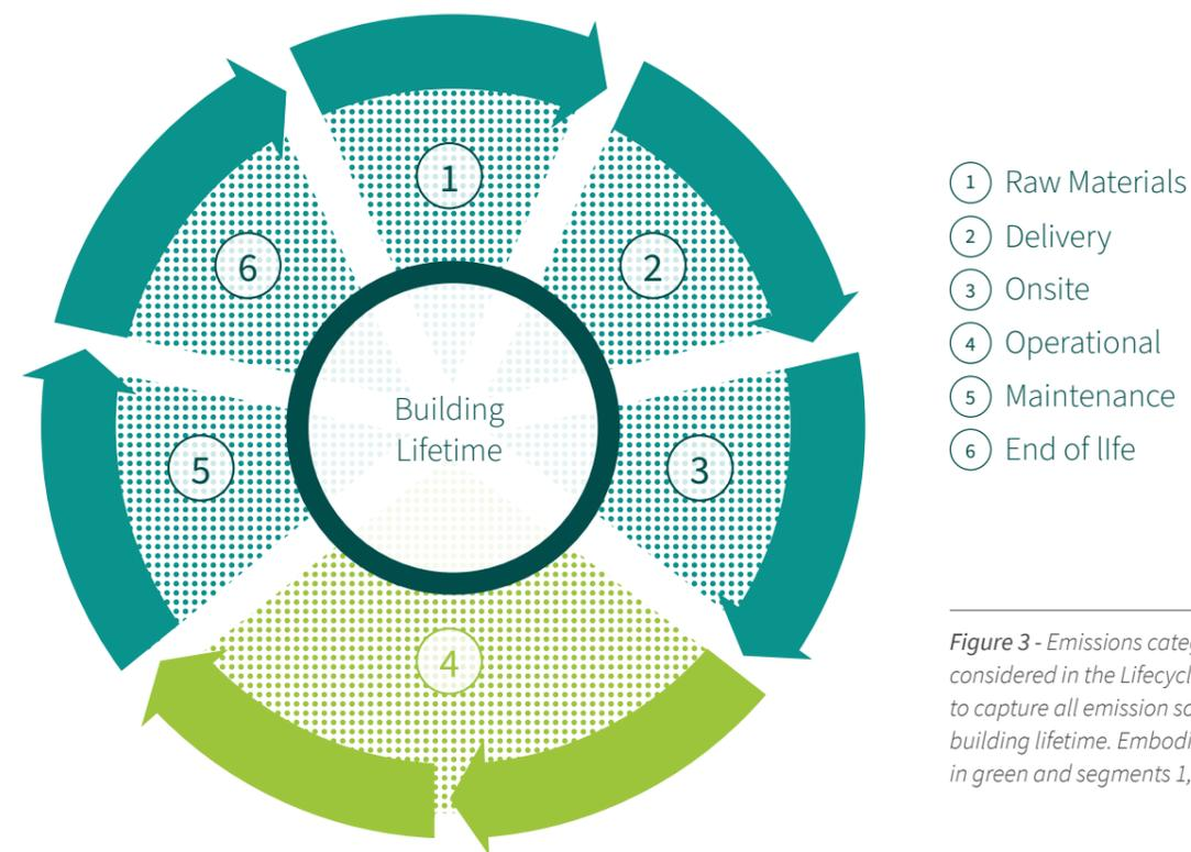
Figure 3 - Emissions category components considered in the Lifecycle Assessment (LCA) to capture all emission sources over the whole building lifetime. Embodied carbon is represented in green and segments 1,2,3,5 and 6.
